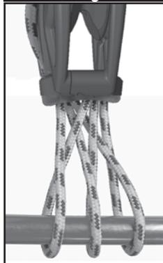
*To lash block at 90° cross lines each pass similar to lashing to boom.*
