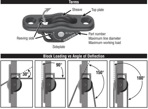
Block load increases when the line turns at a greater angle. Block loads double when the line turns 180°. If there is 400 kg (880 lb) on the line and the angle of deflection is 180°, the Harken throughdeck block is subject to 800 kg (1760 lb). Select blocks carefully. See specification chart on next page.
